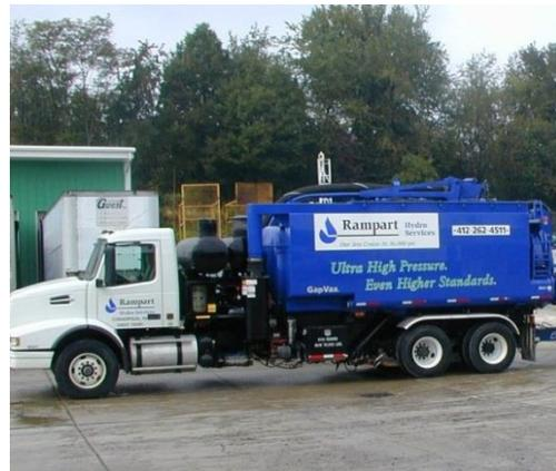
Rampart's wet/dry vacuum trucks are specifically designed to perform hydrodemolition cleanup and wastewater control. The trucks are
